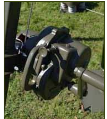
The mast hoist for raising the mast sections has two gears for heavier headloads. The hoist is only reversed by push-button brake with automatic centrifugal descent control.
