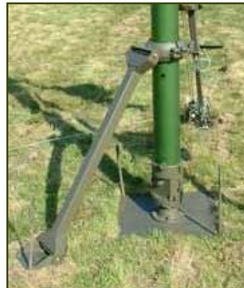
The brake arm assembly secures the mast assembly in the desired direction.
