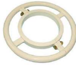
CAT NO. 13272 Wheel Handle This solid aluminium handle is fitted to the 4.5" base tube of the PT mast when rotation is required. Weight: 1.16Kg
