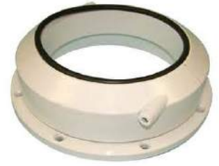
CAT NO. 14048 Roof Bearing Used when fitting a PT mast through the roof of a vehicle allows 360 degree rotation and is fitted with PTFE bearings and a weather proof ring. Weight: 1.26kg
